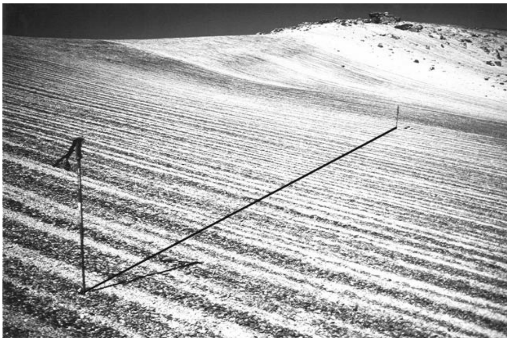
Figure 2 Method for measuring the spacing distance of stripes from a fixed line. Cerro Visuya, 5200 masl.
